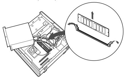
The memory modules are located beneath the power supply.
